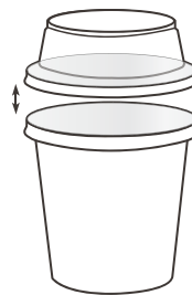
Seal-in: Double vertical compartment: seal on the lid and seal in the tray.
